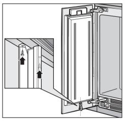
■ From below, screw the air separator firmly onto the door with the 2 screws.
